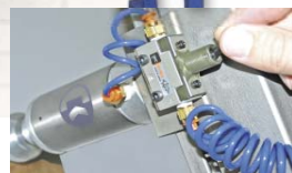
Each cylinder can be actuated individually or all at once with a master switch
